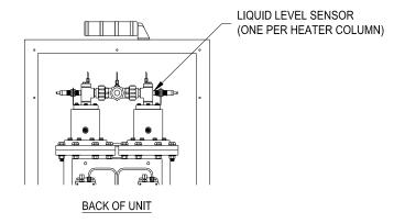
Figure 42: Liquid Level Sensor
