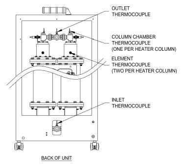
Figure 43: Thermocouple Locations
