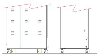
Figure 8: Seismic Brackets (top-half) Attached to Cabinet
