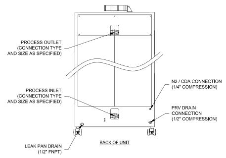
Figure 10: Water, Gas Plumbing Connections
