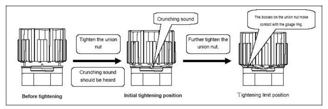
Figure 13: Super 300 type Pillar fittings tightening procedure
