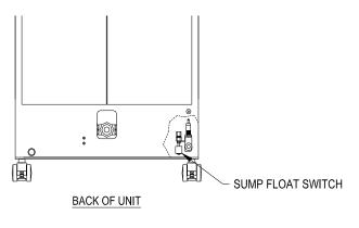
Figure 44: Leak Detector
