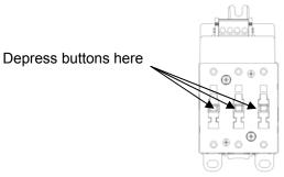
Figure 51: Safety Contactor
