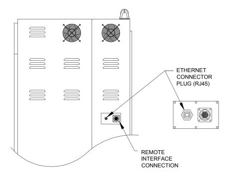
Figure 40: Ethernet RJ45 connector plug
