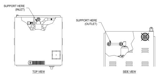
Figure 11: Support Internal Piping when Connecting Plumbing (2-column unit shown)
