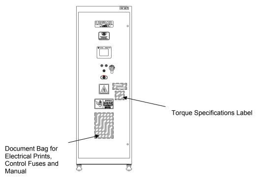
Figure 15: Location of Torque Specifications Label
